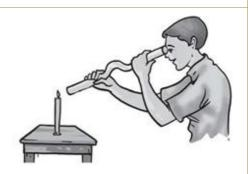
2. Light cannot be seen through a bent tube.
