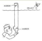
A **periscope** inside a submarine to observe objects outside the submarines.
