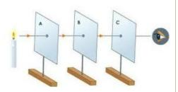
1. The **light** of the candle **can be seen** because all the **holes are in a straight line**.
