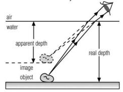
Also, if you put a spoon at an angle in a cup of water, it will appear to bend at the water-air boundary.
